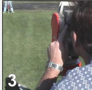
Using the built-in telescopic sight, the LaserLynx operator aligns the unit on the prism held by the marking official.
