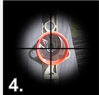
When the LaserLynx prism is at the center of the cross-hairs, the operator taps the **acquire** button on the FieldLynx unit and distance is calculated.
