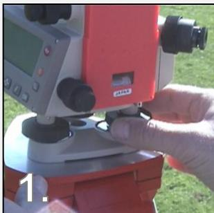
Prior to the event, the LaserLynx unit is set up adjacent to the throwing area and leveled.
